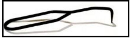
This is a gadget which is used for cleaning out the grooves on the side bars, which are left filled with wax when the old comb is removed.
